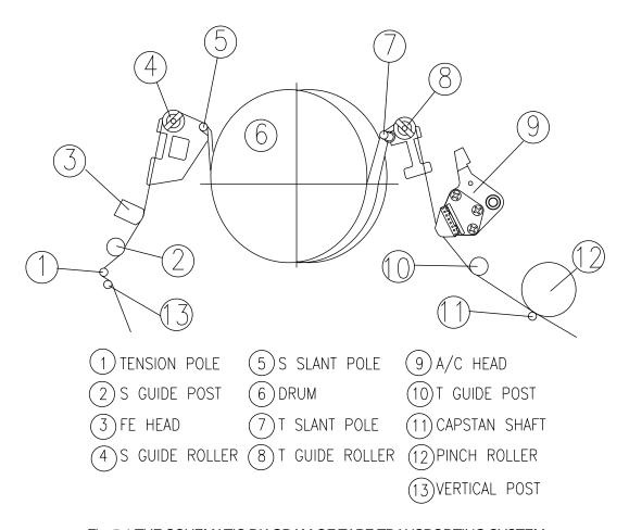
Fig. 5-1 THE SCHEMATIC DIAGRAM OF TAPE TRANSPORTING SYSTEM
